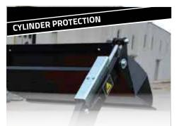
Galvanized sheet, protects the moving parts from materials that could damage them
