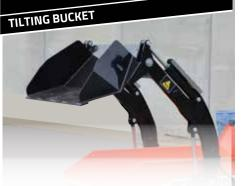
The tilting bucket not only load the dumper but can unload it frontally
