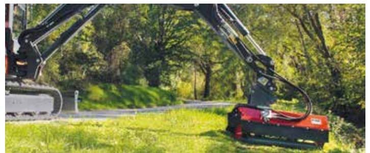
Single/double effect hydraulic system with electrical containment (50 lt/min)
