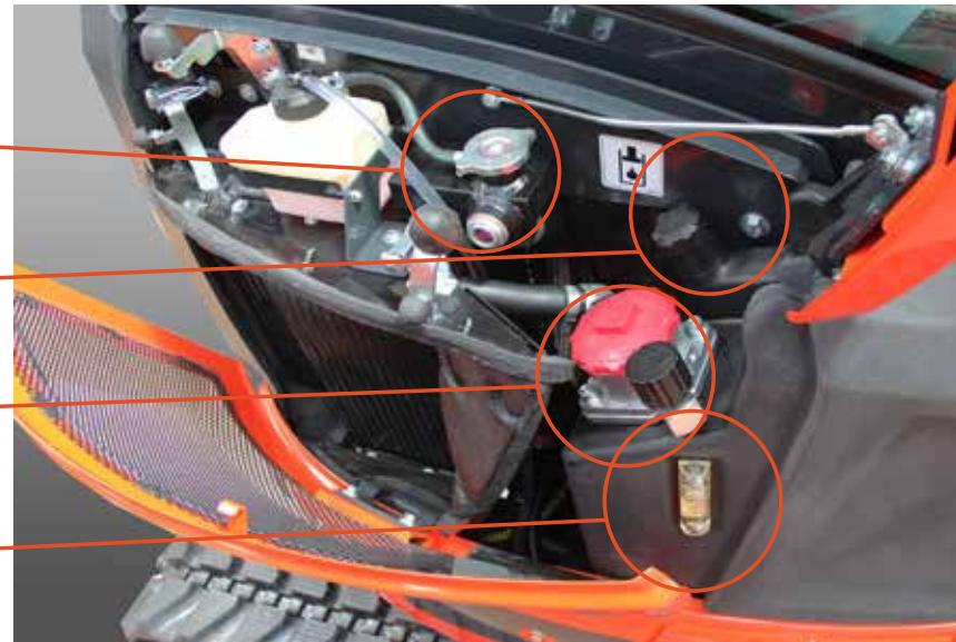
All access points for daily checks and for routine maintenance are concentrated in defined areas, optimizing machine downtime. All elements are easily accessible and located in practical and functional positions.
