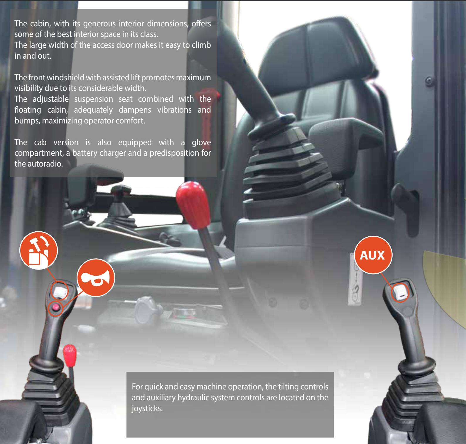
For quick and easy machine operation, the tilting controls and auxiliary hydraulic system controls are located on the joysticks.
