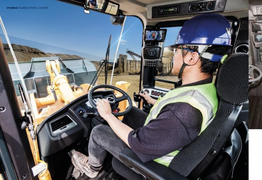
The HL980A has a **large**, **air suspended**, **comfortable seat** with heating as standard. The seat and armrest are fully adjustable.
