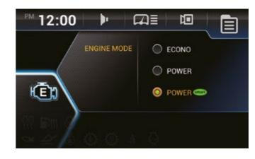
The new **Smart Power mode** adjusts engine RPM in heavy load work like digging to save fuel without compromising on performance. The technology also achieves an optimal balance between traction and breakout forces.
