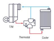
The HL980A is equipped with a **thermostat for transmission cooling**. This feature helps to warm up the fluid quickly and keeps it at the optimal working temperature, protecting components and increasing efficiency.
