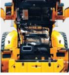
Auto greasing system With the optional auto greasing system, grease is applied to lubrication points automatically when needed. The correct dosing is ensured and lubricant is applied uniformly, reducing grease consumption and eliminating waste.
