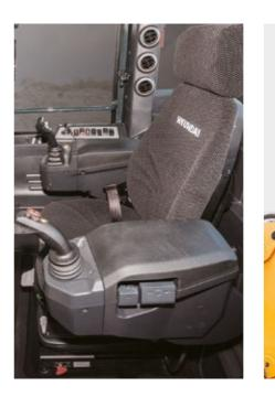
Adjustable seat and armrest The HL975A CVT has a large, comfortable air suspension seat with heating as standard. The seat and armrest are fully adjustable for added comfort.
