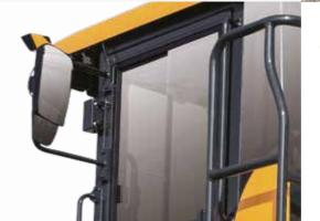
The **side mirror** is easy to adjust for optimal visibility and can be folded away to prevent damage during transportation.
