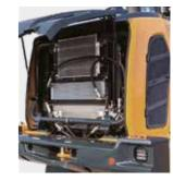
The HL955A has a dependable wide-core and fin air cooler that prevents performance degradation caused by contamination.
