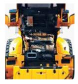
The tilt-back engine hood is fully retractable and can be opened electrically for easy access to the sealed engine room and cooling room. The engine room is designed to prevent the possibility of fire caused by the inflow of foreign materials.
