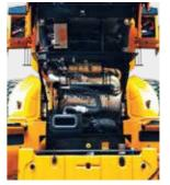
The tilt-back engine hood is fully retractable and can be opened electrically for easy access to the sealed engine room and cooling room. The engine room is designed to prevent the possibility of fire caused by the inflow of foreign materials.
