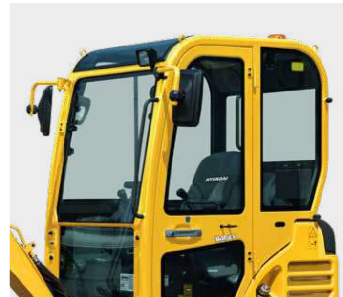
Flat glass The cabin windows and panels are designed with flat glass to allow easy replacement in the event of damage.
