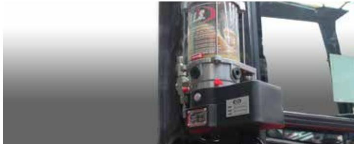
Automatic centralized lubrication
