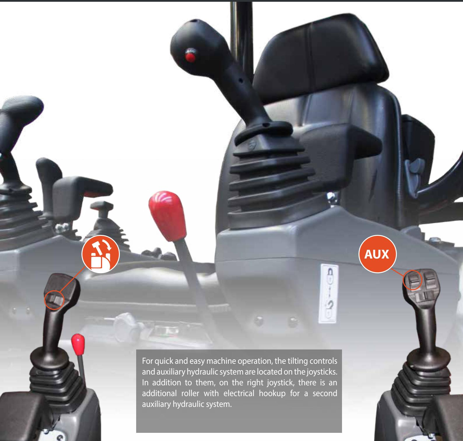
For quick and easy machine operation, the tilting controls and auxiliary hydraulic system are located on the joysticks. In addition to them, on the right joystick, there is an additional roller with electrical hookup for a second auxiliary hydraulic system.
