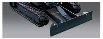
Easier to Transport Four tying-down holes allow easier transportation.
